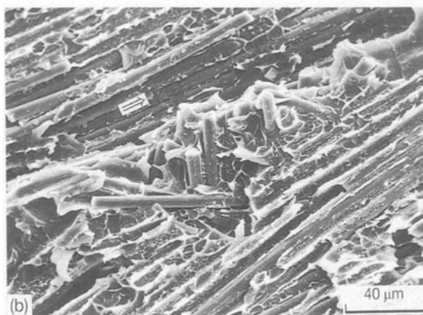
Figure 13 SEM observation of the fracture surface of UD commingled composite. The arrow indicates the direction of crack propagation.
